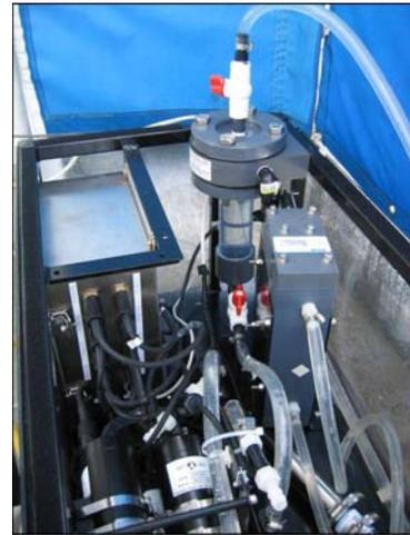
**Figure 1.** *Flow-through system equipped to measure FI-Chl, FI-CDOM, beam attenuation, DO, Temp, and Salinity. Seawater is pumped through the system from below the boat at a rate of 20L/min.*
